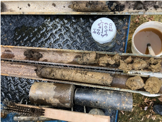
Sample of Fill – Silty Clayey Sand (SC-SM) with gravel
